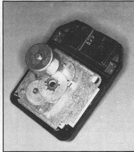
Motor, gears below top plate activate coolant valve, contact arm, vacuum distributor.
